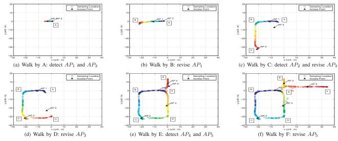
Fig. 4. Illustration of the online co-localization when a user walks from A through B, C, D, E to F.
